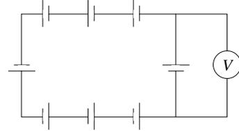
Each battery has an *emf* of 1.5 V and an internal resistance of  $0.2 \Omega$ . What is the reading on a voltmeter connected across any one of the batteries?
