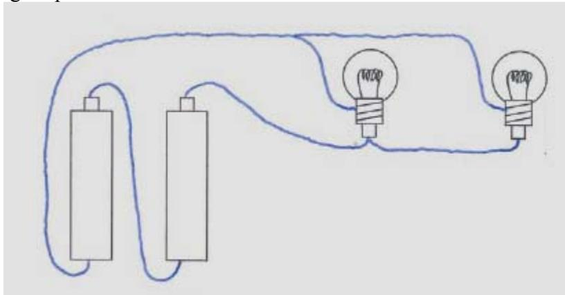
**The batteries should be in series, the bulbs should be in parallel and the wires connecting them to the batteries should be placed on the correct terminals.**
