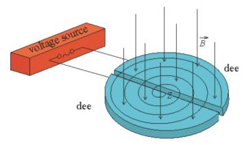
The magnetic field forces the particles to travel in a spiral path. The energy is applied to the particles as they cross the gap between dees in the cyclotron and so the particles are accelerated. This effect increases the radius of the circle and so the path is spiral. With no change of energy, the charged particles follow a circular path. A charged particle will gain its maximum speed when the radius of its path reaches the radius of the cyclotron.
