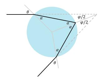
The next step to seeing how this relation results in the primary bow is to plot it. You can see plots of above relation  $\varphi(\theta)$  for the different indices of refraction of red, green, and violet light at desmos.com/calculator/koohasiyly.
