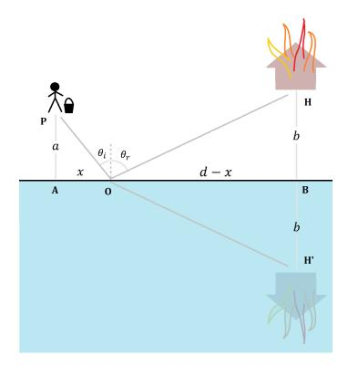
Since the path of least time is the shortest path in this case (there is no change of medium, and hence speed), the  $\overline{POH'}$  resulting in least time is a straight line.
