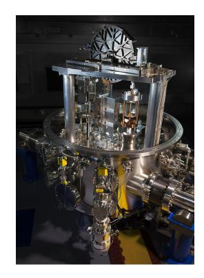
If we write a relationship for a mass that is measured with a kibble balance, we will find that the equation contains the parameters g,  $\varepsilon$ , and I. We can measure g with high precision using an absolute gravimeter while the induced emf( $\varepsilon$ ) and and current (I) can be measured using Josephson's effect and the quantum Hall effect, respectively.
