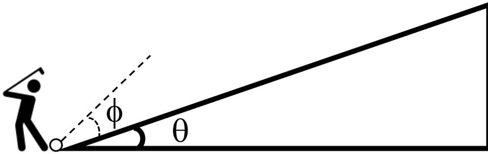
A golfer is playing golf facing an inclined plane of inclination angle  $\theta$  as shown in the figure. When he strikes the ball, the ball flies towards the inclined plane. The ball left the ground at an angle  $\phi$  relative to the inclined plane. What is the value of  $\phi$  at which the ball can land the farthest distance along the incline? Neglect air resistance and assume the inclined plane is infinitely long.
