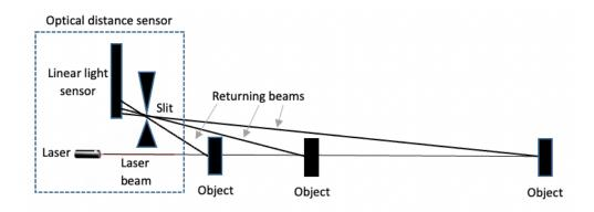
The components inside the dashed line box form the optical distance sensor. The vertical rectangle represents a linear light sensor, which measures the point of impact of the returning beam. The three lines indicate light rays reflected from objects at different distances.
