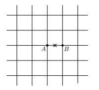
Consider an *infinite* grid made of identical wires of resistance 1  $\Omega$ . The equivalent resistance between two adjacent points A and B is  $R_{AB}$ . If the wire connecting A and B (marked with x) is cut,  $R_{AB}$ :
